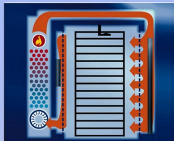
The heat exchange in the gas-fuelled oven is in accordance with the counter-flow principle.
